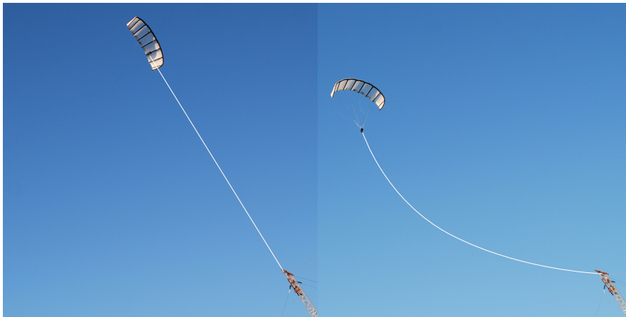
Fig. 7.2: Kite performing crosswind flight maneuvers with practically straight tether while reeling out (left) and non-maneuvering kite with strongly sagging tether while reeling in (right). Photographic footage with traced tether from 2 August 2012.
